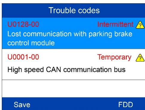
Figure 3-5 Sample ABS Trouble Codes Screen 1
