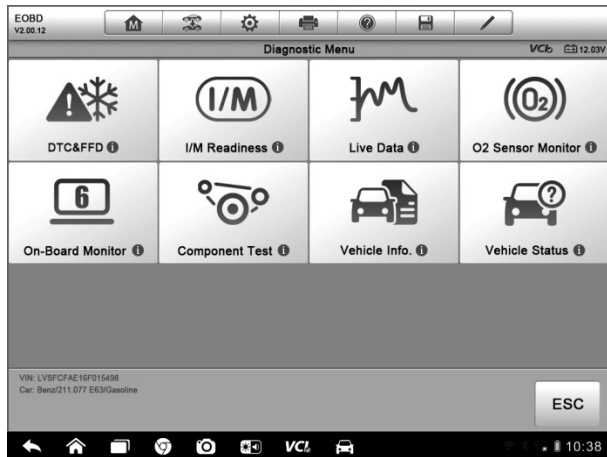
Figure 4-14 Sample OBD II Diagnostic Menu
