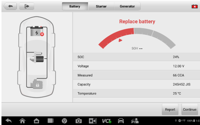
Figure 6-6 Battery Test Results Screen
